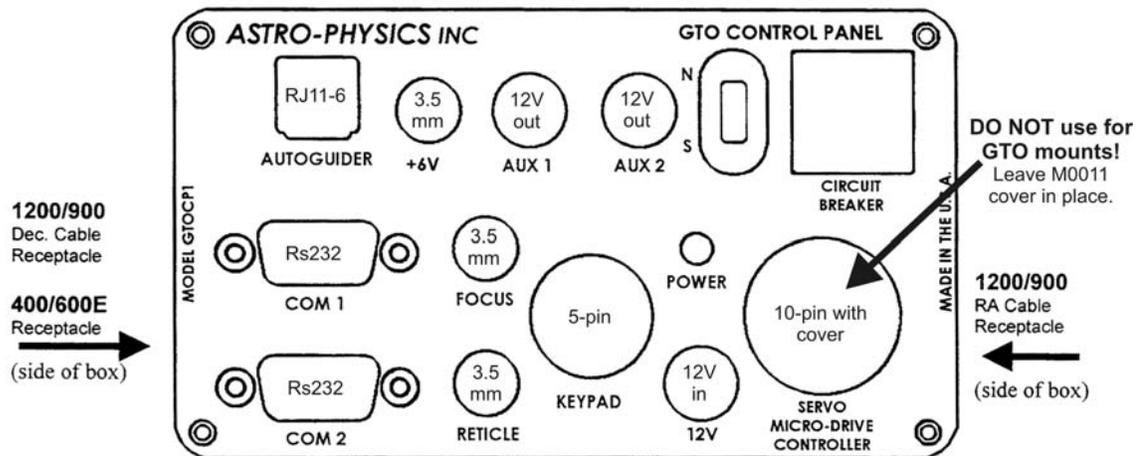
The GTO Control Box is mounted directly onto the polar axis of the 1200 and 900 mounts and is a stand-alone unit for the 400 and 600E mount. Please remember that this box contains advanced electronics and must be treated with the same care given to other fine equipment. Support the stand-alone unit in a secure manner so that it does not fall. Do not place it in the wet grass or dust. You can see that the unit is built to be rugged. However, it is not indestructible.
