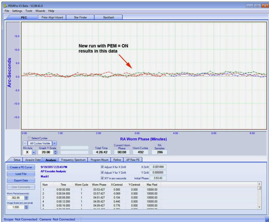
4. Once you have loaded this curve into the controller's memory (CP1 thru CP4), you can now turn on PEM and do one more run of 1 to 3 worm cycles to see how well the mount now tracks.
