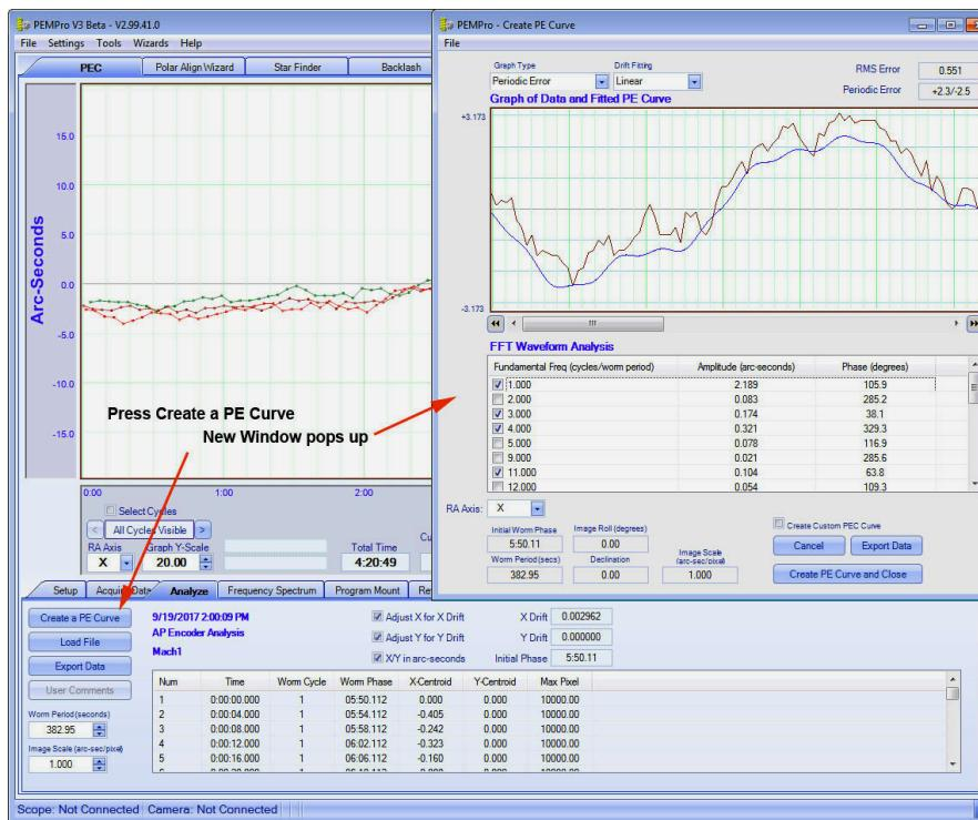
2. Next step is to create a PE curve from this data. Press the button to create new PE curve. A new window will pop up which shows a basic fitted curve with the major harmonics and their values.
