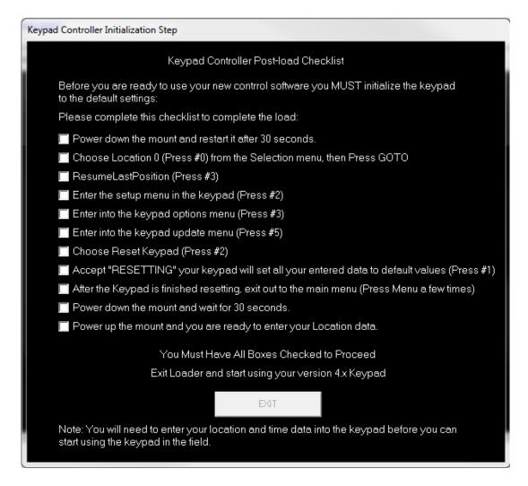
10. Your GTO keypad is now updated to the new EPROM code and is ready to use. Turn the power to the control box off, wait 30 seconds, then turn back on. If the location selection screen comes up first, enter 0 and press GOTO. Then, press ResumeLastPosition to get to the Main Menu.
