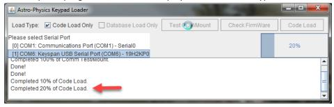
8. When the upload is complete, the Keypad will beep once and display the new version number. The computer dialog box will indicate that the process is "Done!". Cycle power to the mount and begin your session.
