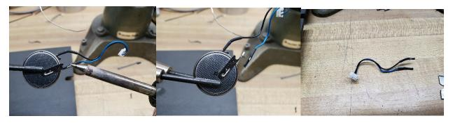
4. If you have heat shrink tubing, now is the time to put it on the wires. Cut two pieces of tubing about ½" (~1 cm) long and slide each one onto the end of a wire until it is at the plastic connector.
