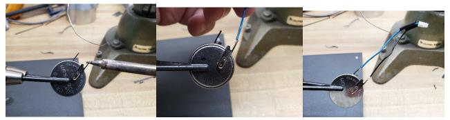
6. After cooling, slide the heat shrink back down the wire and press it onto the tab. You can use the soldering iron to gently warm and shrink the tubing down on the connection, but a heat gun will work better.
