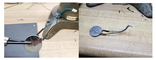
The replacement is now complete, and you are ready to install the battery into your keypad.
