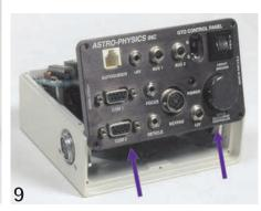
**5.** Push in the 2 cable connectors on the sides as shown in diagram 8.
