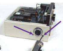
**3.** Remove the 2 screws on each side of the control box near the cable connector. This is shown in diagrams 4 and 5.
