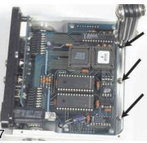
**4.** Use a 7/64" Hex Key to loosen and remove the 3 hex key screws from the back of the control box. This is shown in diagrams 6 and 7.
