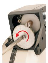
Remove the cover to expose the clustered spur gears beneath. The worm's spur is hidden underneath the large spur gear that is on top of the cluster. This top cluster gear must be removed.
