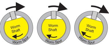
Correct - Tight Set Screw Centered on the Flat Spot on the Worm Shaft Causes Worm to Turn with Spur Gear
