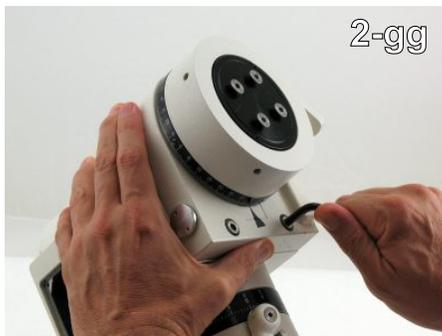
Step 40 Push the worm housing up against the worm wheel and put the two M6 SHCS and washers back into place. Tighten lightly. (2-gg)
