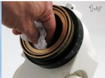
Step 12 - Once apart, the inside bore of the worm wheel can be cleaned and greased with Lubriplate 105. (1-u, 1-v)
