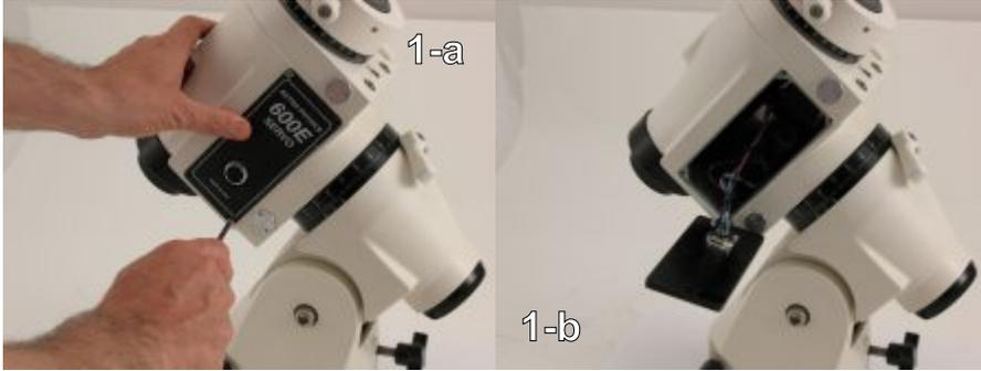
Step 1 - Remove the mount nameplate using a Phillips-head screwdriver. (1-a,1-b)
