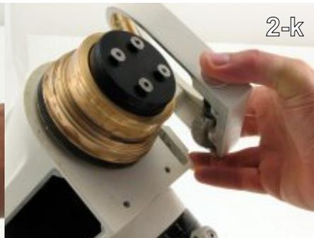
Step 24 - With the 5mm hex key, remove the two M6 x30mm SHCS and washers from the worm housing. Carefully remove the worm housing from the assembly. (2-j, 2-k)
