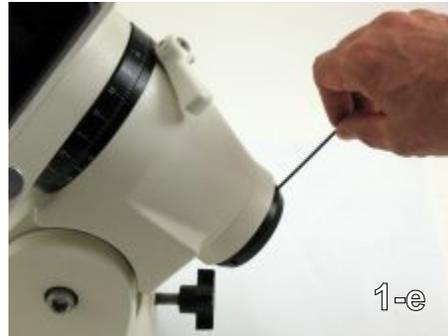
Step 3 - Using a 2mm hex key, back off all three of the M4x6mm brass tipped socket set screws retaining the pre-load ring. Please note that several rotations of the screw will be necessary as the brass tip of the screw is in a groove cut into the shaft approximately 1mm deep. (1-e)
