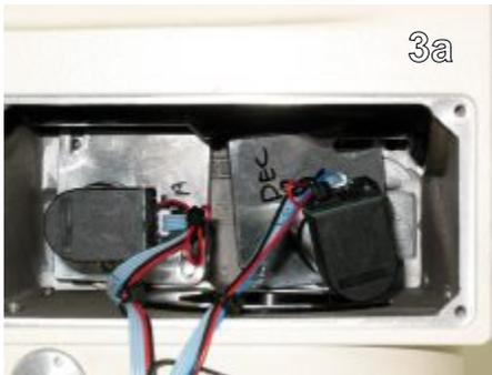
Step 44 - Place the motors back into the declination/motor housing. The right ascension motor is in the bottom position and the declination is on top. If you failed to mark which is which, plug them into your controller and the right-ascension motor will be the one in continuous rotation. (3a)
