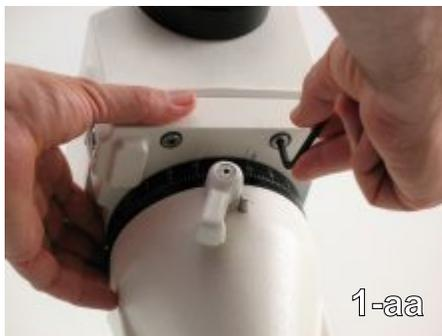
Step 16 - Put the two M6 x 30mm SHCS and washers back in the worm housing and tighten lightly. (1-aa)
