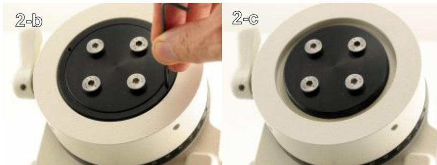
Step 20 - Remove the thin ring at the top of the declination shaft by rotating it. Use a 2mm hex key in one of the two holes provided. (2-b,2-c)
