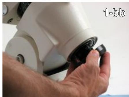
Step 17 - Return the pre-load ring to the rear of the RA shaft and rotate it until it makes contact with the rear bearing. Then, back it off approximately 1/8 turn or 15-20 degrees. Lock down all 3 screws as evenly as you can. (1-bb)
