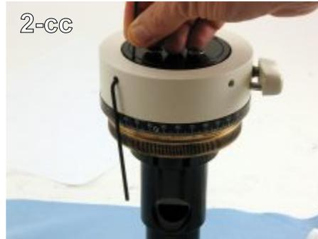
Step 37 Firm up the torque on the 4 set screws and tighten the thin ring. (2-cc)
