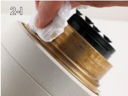
Step 23 Remove the old grease from the outside diameter of the worm wheel and replace with the Lubriplate 105. (2-l)
