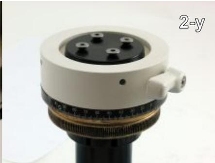
Step 33 - Make certain that you put the small brass disk back in the painted clutch knob ring before mounting it onto the worm wheel. Rotate the ring to place the clutch knob in the same orientation that it was in before disassembly. (2-x, 2-y)
