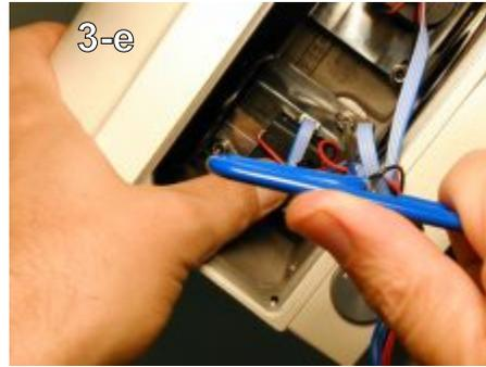
Step 47 - There is no need to press the motor spur gears tight against each other before applying final torque to the screws. Light finger pressure is all that is required. (3-e)
