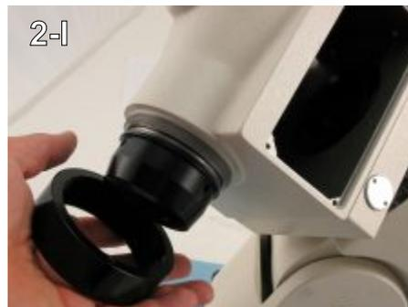
Step 25 - Unscrew the encoder adapter ring from the declination/motor housing. (2-l)
