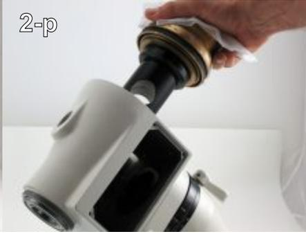
Step 27 - Push up from the bottom, (counterweight side) to remove the declination shaft and worm wheel from the housing. (2-o, 2-p)
