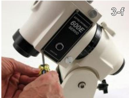
Step 48 - Put the name plate back in place. Position the wires so that they do not block the use of your polar scope. Return the two sight hole screws, if you removed them in step 46. (3-f)
