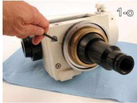
Step 9 - With the 5mm hex key, remove the two M6 x30mm socket head cap screws (SHCS) and washers from the worm housing. (1-o)
