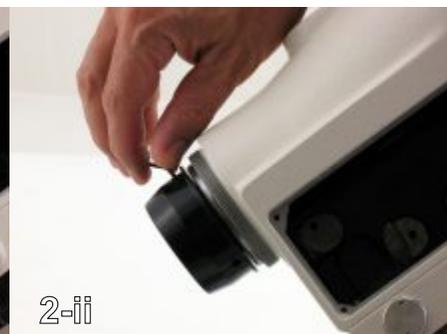
Step 41 - Return the pre-load ring to the rear of the declination shaft and rotate it until it makes contact with the rear bearing. Then, back it off approximately 1/8 turn or 15 - 20 degrees. Lock all 3 screws down as evenly as you can. (2-hh, 2-ii)
