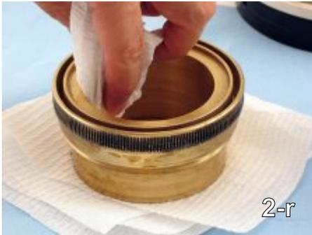
Step 29 - Once separated from the shaft, clear the old grease from the bore of the gear and lubricate with Lubriplate No. 105. (2-r)
