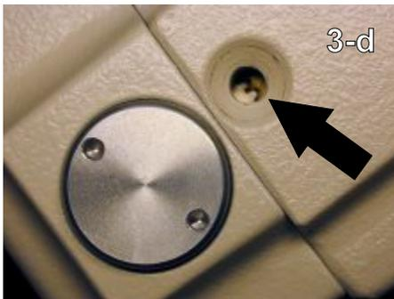
Step 46 - You can verify that engagement has been made by removing the slotted screw on the opposite side of the declination /motor housing. (3-d) This opens a sight hole providing visual proof of gear tooth engagement. There is one for each axis.
