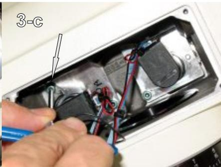
Step 45 - Position the motors so that the brass idler gear contacts the stainless worm spur gear that you turned with your fingertip earlier. Using the 3mm "T" handle hex key, lightly engage all four mounting screws and washers. Don't forget to engage the ground wire under one of the right ascension mounting screws. (3-b, 3-c)
