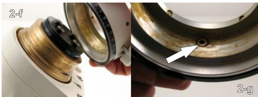
The small brass disk should be fished out with the 2mm key before it falls out. Do not clean it as the grease is used to hold it in place for reassembly. (2-d, 2-e, 2-f, 2-g)
