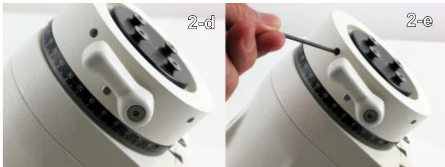
Step 21 - Release the tension on the declination clutch knob. Using a 2.5mm hex key, back off the 4 brass tipped set screws in the painted ring. The declination setting circle is attached to the ring. Lift the ring off the top of the declination shaft.
