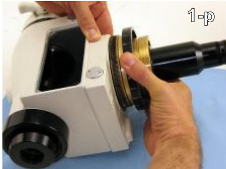
Step 10 - Push the worm housing down (towards the counterweight shaft connection). Pull the worm wheel off the right-ascension shaft. If you have a problem, go to step 10A. (1-p)
