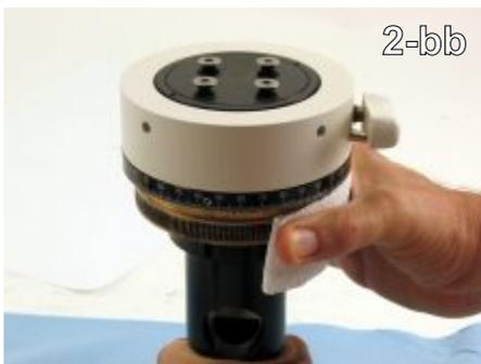
Step 36 - To check that you have assembled this part correctly, hold the shaft and rotate the worm wheel gear. It should turn easily with a little more drag than when the gear was first put in place in step 32. If not, back off the 4 screws from Step 35 and re-tighten evenly or go back to step 34 and back off the pressure on the ring. (2-bb)
