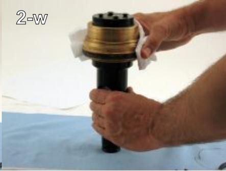
Step 32 - Stand the declination shaft on the counterweight end. Place the worm wheel gear back on the declination shaft and give it a few rotations. (2-v, 2-w)
