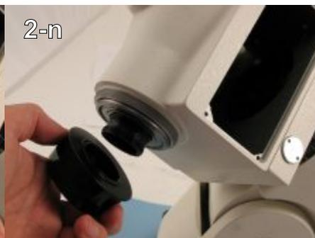
Step 26 - Using a 2mm hex key, back off all three of the M4x6mm brass tipped socket set screws retaining the pre-load ring. Please note that several rotations of the screw will be necessary, as the brass tip of the screw is in a groove cut into the shaft, approximately 1mm deep. Remove the pre-load ring. (2-m, 2-n)
