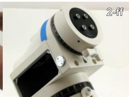
Step 39 Return the finished declination shaft assembly to the declination/motor housing. (2-ee, 2-ff)
