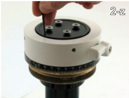
Step 34 - Place the thin ring, removed back in step 20, into place and rotate it down to a stop. Tighten very lightly. (2-z)
