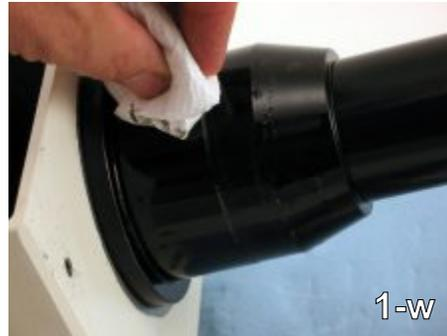
Step 13 - Do the same with the exposed right ascension shaft. (1-w)
