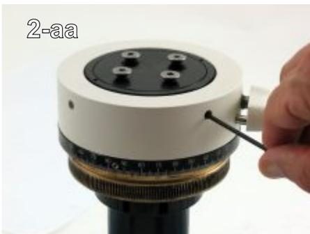
Step 35 - Make certain that the clutch knob is loose. Use the 2.5mm hex key to tighten up all four of the socket set screws in the painted clutch ring. It is important that the torque applied to each screw be even. The thin ring will hold the clutch ring in place to keep it from lifting up. (2-aa)
