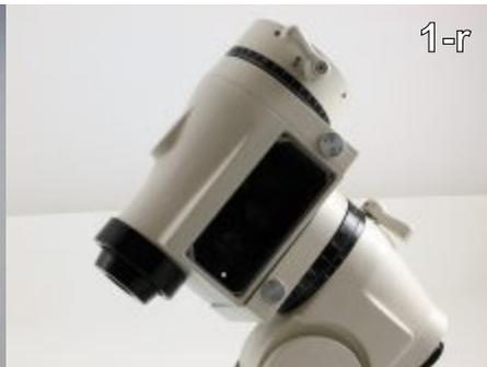
Step 10A - If step 10 proves to be difficult, you can avoid damage by placing the small brass disk back under the clutch knob and putting the assembly back into place. Now the clutch knob can be tightened to hold the worm wheel and you can pull the shaft out of it. (1-q, 1-r)
