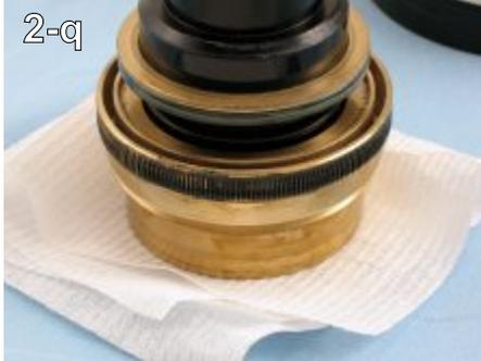
Step 28 - Turn the shaft upside down and let gravity release the worm wheel from the shaft, if possible. (2-q)
