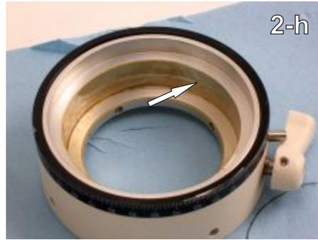
Step 22 Clean the old grease from inside the painted ring and replace with Lubriplate 105. (2-h)
