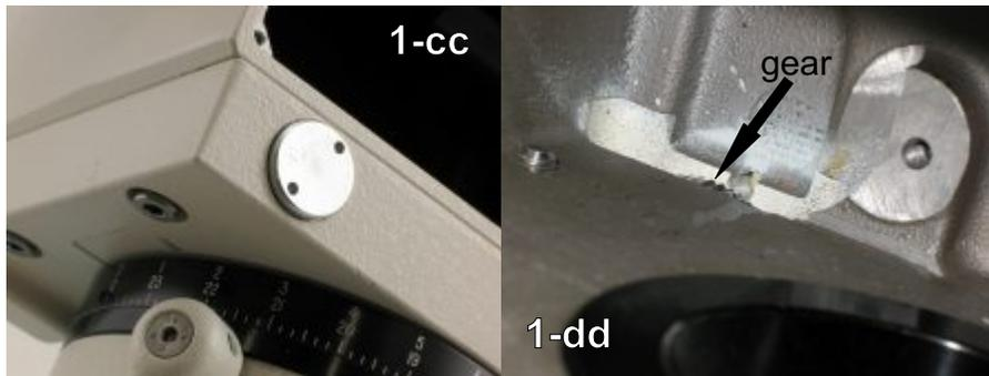
Step 18 - Since you have disassembled everything, you will need to align the worm housing so that it is squared up with the declination/motor housing. Apply some pressure to the worm and lock down the two mounting screws. With no motors in place, adjust the tightness by placing your hand into the housing and rotating the right ascension worm spur with your fingertip. Once no backlash is present and the spur gear turns with your finger, you are done. (1-cc, 1-dd)
