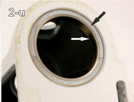
Step 31 - Clean and lubricate the counterweight side of the shaft and ring, plus the bearing surface machined on the top of the declination/motor housing. (2-t, 2-u)
