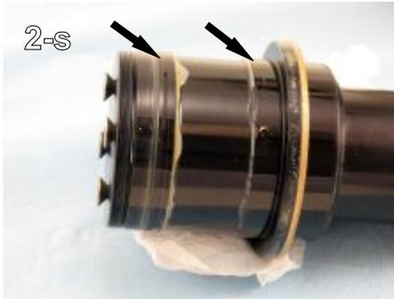
Step 30 - The same is done for the contact surfaces of the shaft. (2-s)
