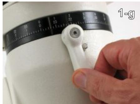
Step 5 - Release the tension on the clutch knob. It is not necessary to undo any of the screws in the knob.(1-g)
