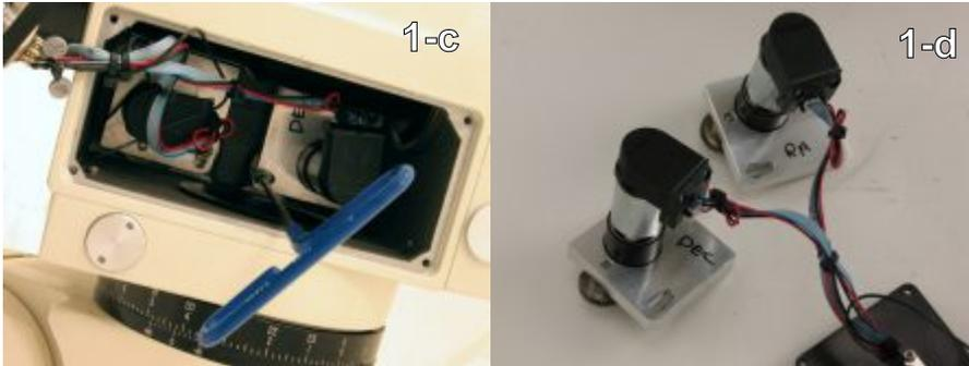
Step 2 - Remove the right-ascension and declination motor using the 3 mm "T" handle hex key. Mark each motor as to their position or axis. Take note of the ground wire on the top side of the right-ascension motor bracket. (Black wire with mounting tab.) (1-c, 1-d)
