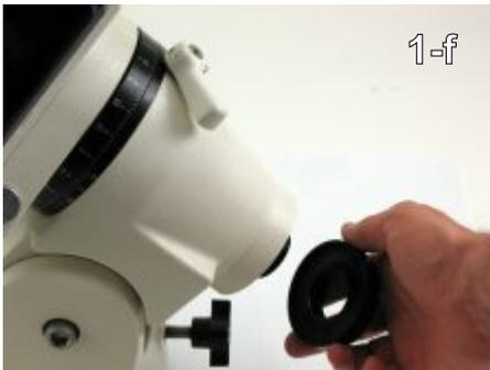
Step 4 - Remove the pre-load ring. (1-f)
