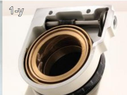
Step 14 - When you are ready to reassemble, put the worm wheel back in the housing if not already there. Don't forget the brass ring! Place the worm housing onto the wheel as shown, fully engaging the teeth. (1-x,1-y)
