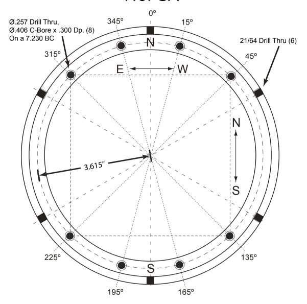
The drawing above provides the necessary detail to drill and tap your flat surface to accept the 119FSA Flat Surface Adapter for 1100GTO and 900 mounts (all versions). The eight counter-bored 1/4"-20 thru-holes are all on a 7.230" bolt circle (3.615" radius). The adapter's full diameter is 8.375". Use 1/4"-20 x 5/8" or 3/4" socket head cap screws to secure the 1612FSA to the flat surface.
