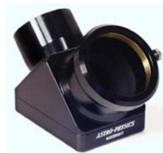
**Reflectivity** - Reflectivity is above 99% over the entire 4000 to 7000 Å photo-visual range. Thin film coatings have extremely low surface scatter compared to aluminum or enhanced aluminum coatings. Examination with a laser source shows approximately a 5-fold reduction in surface scatter.
