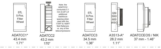
Spacing from the rear surface of 175FF and 160FF when Backfocus Spacer Extensions are removed:
