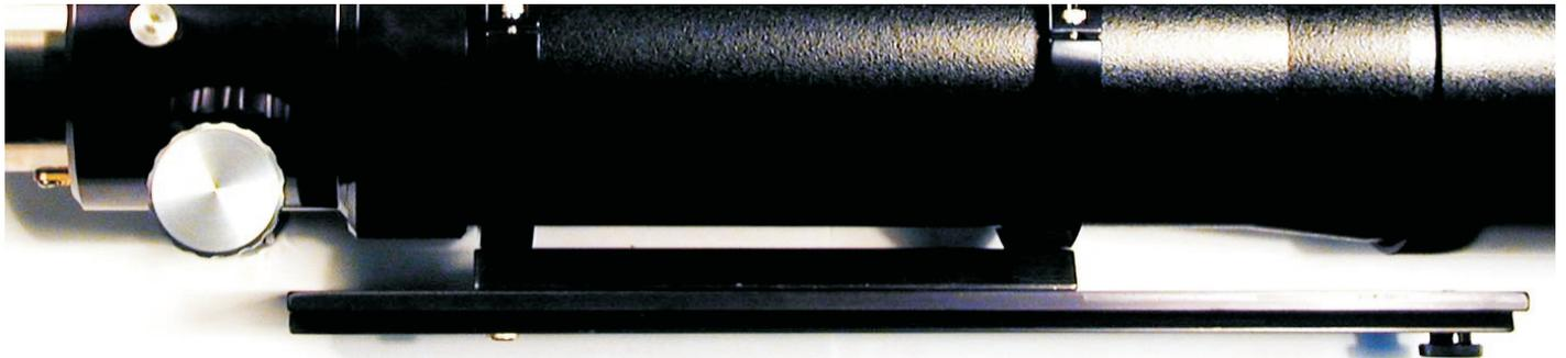
To use the Traveler or the Stowaway with a Losmandy "D" series dovetail plate you will need a 13.5" Losmandy Universal Plate (LMDUP) and an Astro-Physics 7" Sliding Bar (SB0800). Since Traveler is short and the Losmandy plate is long, you will need to add the 7" sliding bar between them as a riser.
