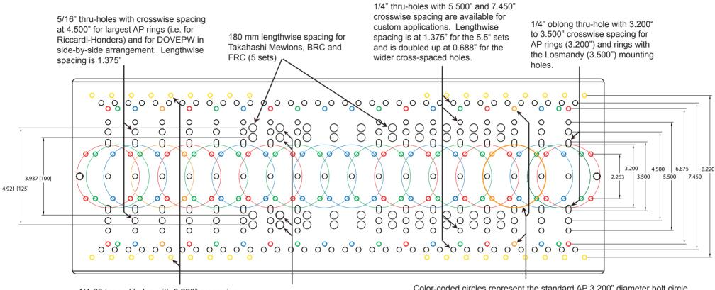
1/4-20 tapped holes with 8.220" crosswise spacing used for locking SB3627 to the DOVE3622 for extra rigidity and security. Lengthwise interval is 1.000".
