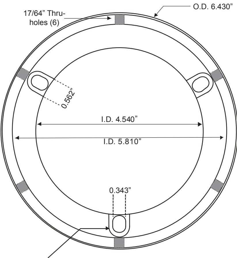
3 Slots spaced 120° apart for 5/16" x 5/8" or M8 socket head cap screws on a 5.110" bolt circle.
