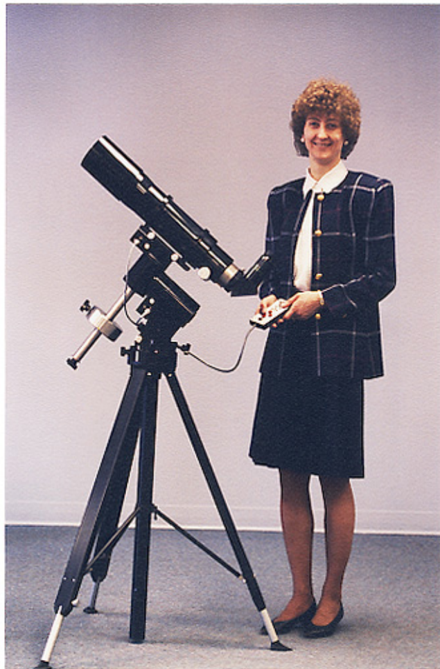
105mm Traveler EDF, 400 German Equatorial with Encoders, Adjustable Aluminum Tripod and other accessories
