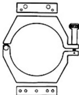
holes for guidescope rings and piggyback camera bracket
