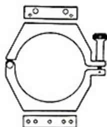
holes for guidescope rings and piggyback camera bracket
