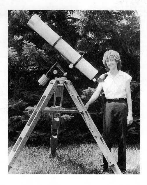
ASTRO-PHYSICS proudly announces a modern Refractor Telescope for serious amateurs. Our new 6 inch F9 Apochromat uses the award winning CHRISTEN TRIPLET design. The objectives are computer optimized for high power as well as wide field photo-visual work. A host of accessories is available to enhance the versatility of this powerful instrument. The result is a limited production telescope with magnificent optical performance, second to none in its class.
