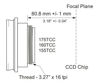
Note: The distance must be the optical distance - not the mechanical distance. Be sure you have accounted for the indexing effects of your filters. [Rule of thumb: add 1/3 of the filter thickness to the adapter length.]
