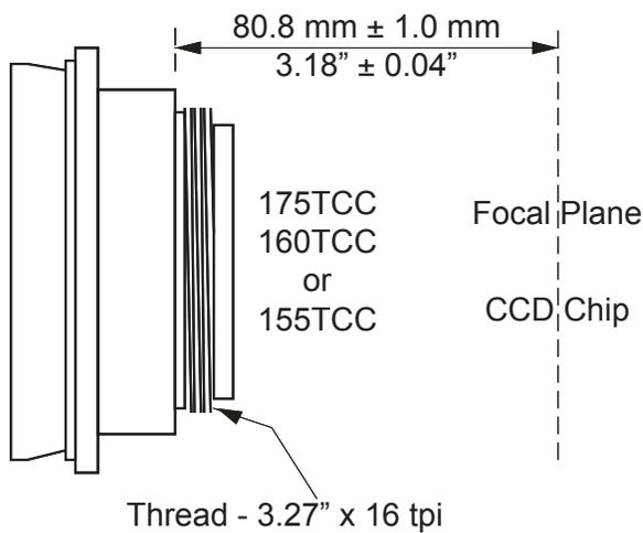
**Remember:** the distance must be the **OPTICAL** distance - **NOT** the mechanical distance. Please be sure that you have accounted for the indexing effects of your filters, sensor window and any other glass in the light path.
